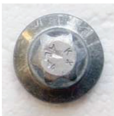
b) Recommended – Outer torx, flange head.
